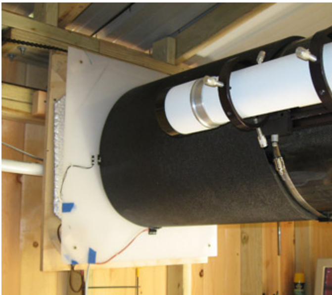
Figure 4: Telescope in its parked position pointed at the flat panel showing proximity sensors.
