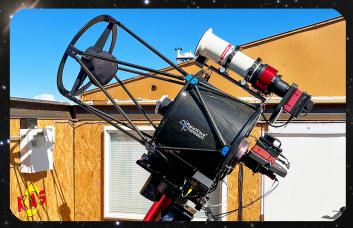
A 20-inch PlaneWave CDK telescope and a 4-inch Takahashi refracting telescope, both outfitted with identical full-frame CCD cameras, make up the KAS Remote Telescope.
