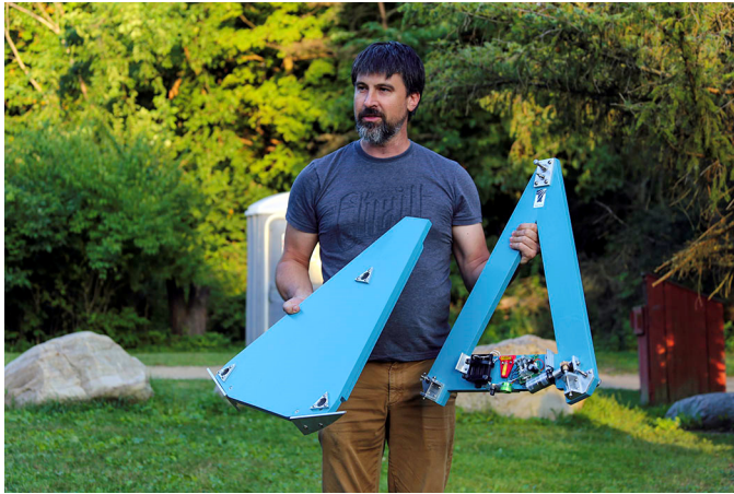
Aaron Roman built this motorized Dobsonian tracking platform that he still needs to try out!
