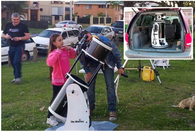
The Board agreed to purchase a Sky-Watcher 8-inch Flextube Dobsonian, similar to the one shown above, at the Oct. 17 th meeting. It will primarily be kept in Owl Observatory and used during public and member-only sessions. However, as its name suggests, the tube can be collapsed for easy transport in most vehicles on special occasions (see inset).
