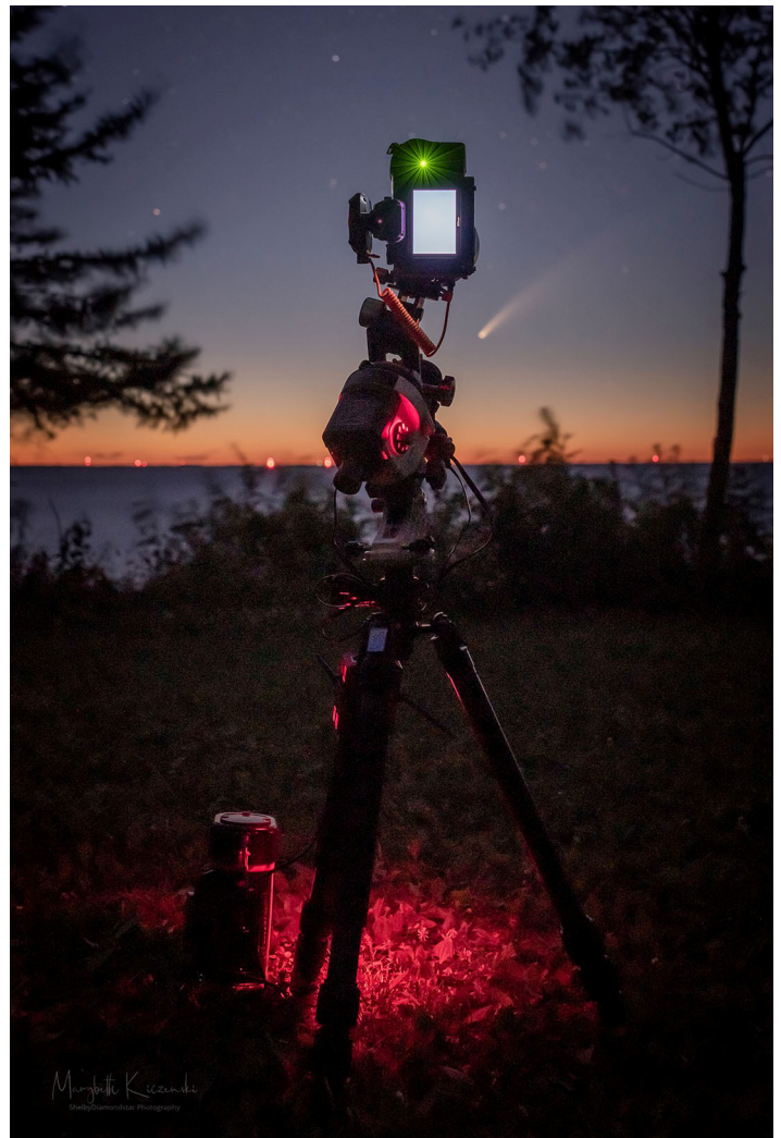
A Nikon Z6 mirrorless camera on a Sky-Watcher Star Adventurer 2i star tracker was used to capture an image of Comet C/2020 F3 (NEOWISE) from Door County, Wisconsin, after sunset on the shore of Lake Michigan in July 2020. The image above was taken with a Nikon D850 camera and Sigma Art 35mm lens. Image courtesy of Marybeth Kiczenski, Shelby Diamondstar Photography ( shelbydiamondstar.com ).
