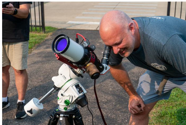
Matt Borton meticulously examines prominences that are dancing along the solar limb using his Lunt 60mm hydrogen-alpha telescope, which is mounted on a Sky-Watcher Star Adventurer GTi.
